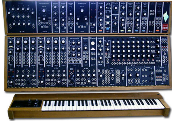
Figure 5: The Famous Moog Modular system
